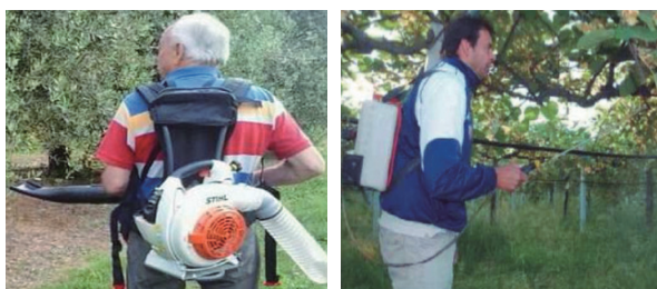
c. Backpack dry pollen pollination blower [68] d. Backpack liquid pollen pollination diaphragm pump [68]
