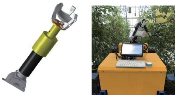
Figure 15 Tomato picking robot end-effector and its whole machine experiment
