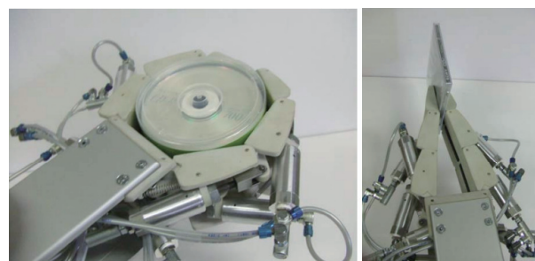
Figure 23 Pneumatically driven robotic wrapped grip and gripping grip
