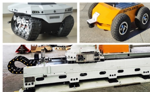
Note: Row 1 presents the crawler and universal wheeled robot bases.
