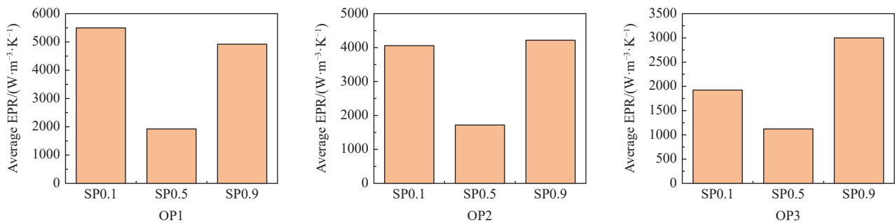
Figure 8 Comparison of average entropy production rate for different spanwise surfaces in runner channel
