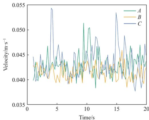
Figure 11 Curves of virus-free potato minituber speed changing with time under different type hole types
