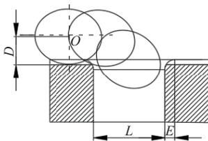
Figure 4 Kinematics analysis of virus-free potato minituber filling the length of type hole
