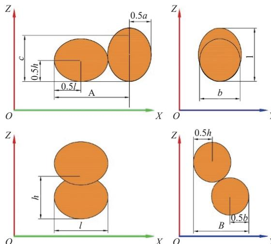
Figure 7 Diagram for calculating the size of the type hole
