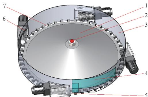
1. Conical turntable 2. Transmission shaft 3. Outer baffle of seed-metering device 4. Baffle 5. Seed outlet 6. Seed cleaning device 7. Type hole
