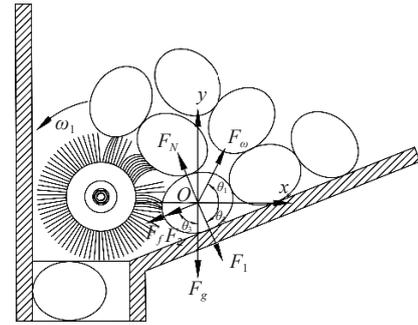
Figure 5 Force analysis of brush cleaning device
