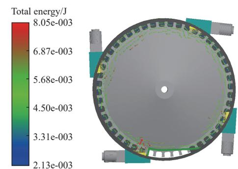
Figure 13 Energy variation of virus-free potato minituber in seed-metering device
