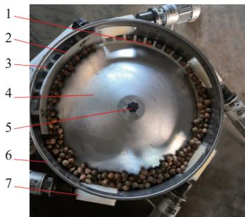
1. Type hole 2. Baffle 3. Seed outlet 4. Conical turntable 5. Transmission shaft 6. Outer baffle of seed-metering device 7. Seed cleaning device
