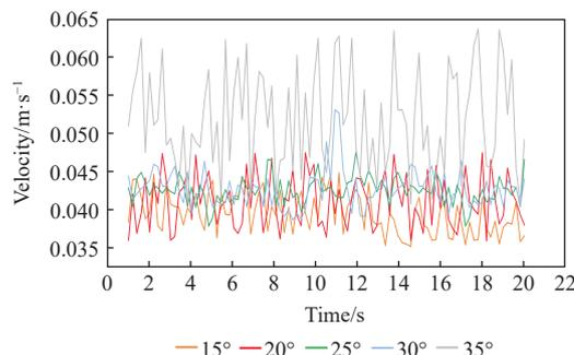
Figure 16 Curves of virus-free potato minituber velocity versus time under different cone disc angles
