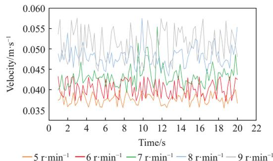
Figure 15 Curves of virus-free potato minituber speed versus time under different cone disc speed
