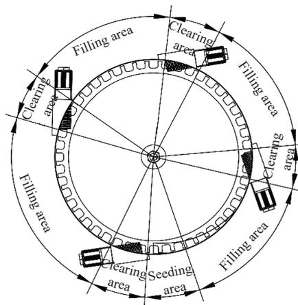
Figure 2 Working principle diagram of the seed-metering device
