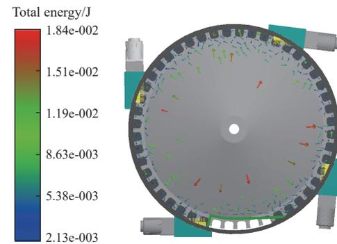
Figure 12 Energy diagram of miniature potato in seed-metering device
