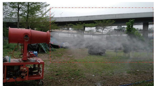
Figure 1 External airflow field of the air-blast sprayer
