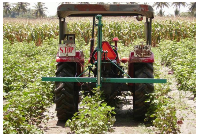
Figure 3 Tractor operated cone penetrometer
