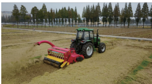
Figure 17 Field verification test of uniform-throwing planter
