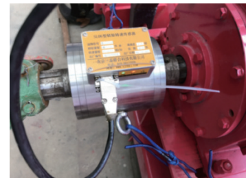
Figure 13 Torque and revolution speed sensor
