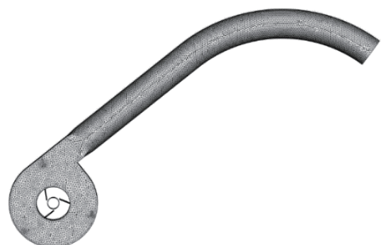
Figure 5 Pipeline grid division diagram of crushed straw lifting and throwing device model
