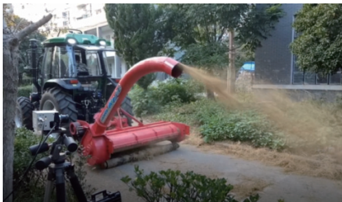
Figure 12 Experimental scenario to verify crushed straw throwing
