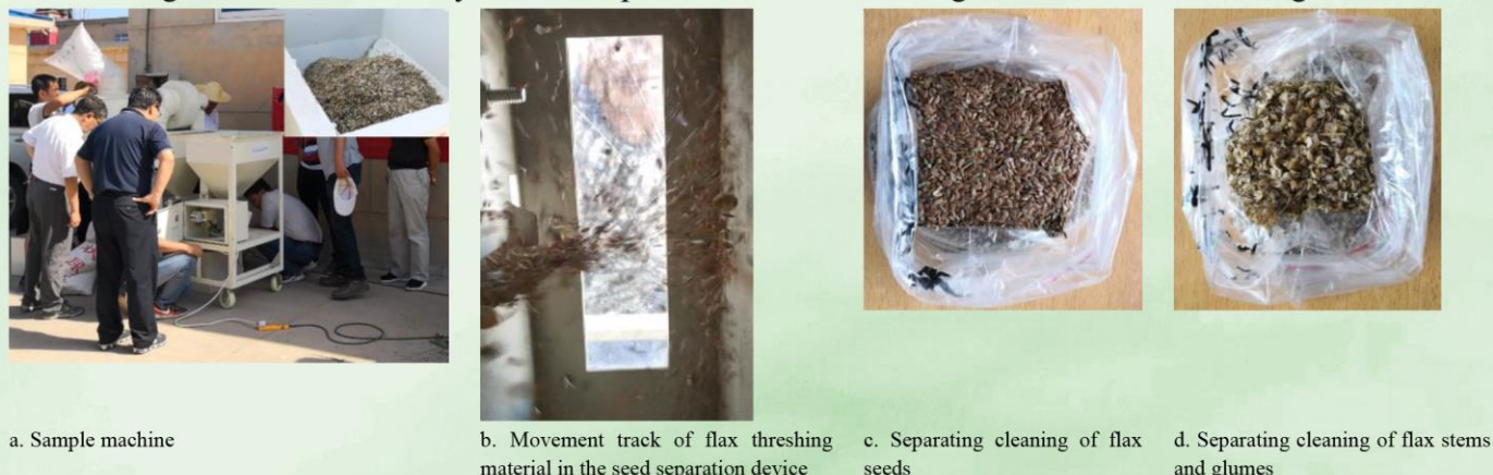
Figure 11 Verification test on the separating cleaning device for flax threshing material
