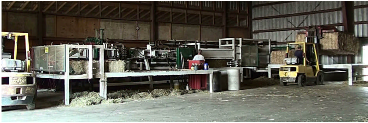
Figure 4 Commercial large square bale compressor (Heidel Hollow Farm, Germansville, PA)
