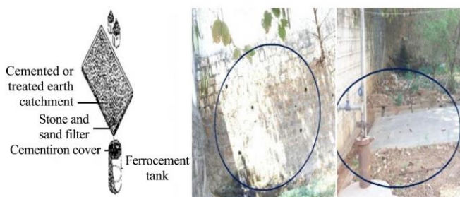
Figure 5 Ground catchment system
