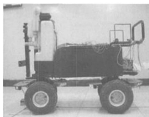
Figure 10 Spraying robot guided by electromagnetic induced line
